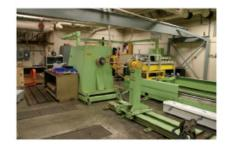
This dedicated low lab space equipped with environmental controls houses a McClean Anderson 5-axis CNC filament winding machine. The system is capable of processing parts up to 66 in. in diameter and 40 ft long using both wet winding and pre-impregnated fiber tows. The winding machine has been modified with a specially designed fiber payout system to enable processing of high modulus graphite fibers with minimal fiber damage.
