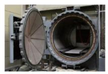
A dedicated autoclave, manufactured by American Autoclave, is used to cure composite structures. The fully programmable autoclave is rated for 650° F, 250 psig, and can process composite parts up to 7 ft in diameter and 11 ft long. The autoclave can process a range of materials including epoxies, cyanate esters, BMIs, some lower temperature polyimides, and thermoplastics.
