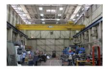
Two 25 ton overhead cranes for main high bay area, additional 25-ton overhead crane for machine shop, smaller 3-ton crane in auxiliary machine shop.
