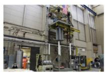
The primary hydraulic composite assembly press in the high bay is 40 ft tall and is capable of generating forces in excess of 500 tons with room for 20 – 25' parts and a 60 in. stroke, one smaller 200-ton H-press with 13 in. stroke, one smaller 200-ton hydraulic four-column assembly press.
